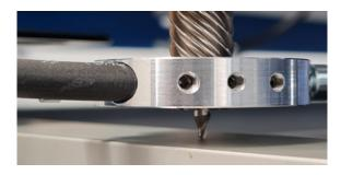
An additional support unit for glass-glass modules offers quick and reliable testing without bending the modules.
