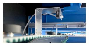
The system can be extended with an automatic cell measurement to measure cells and their geometry with an additional back light image. This includes cell gap measurement, measurement of the interconnection area, controlling of the interconnection area for foreign materials and the inspection of the cell edges.
