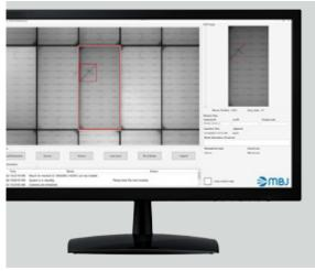
Defective cells will be marked and classified for easy identification. The overall quality of the module can be graded accurately.
